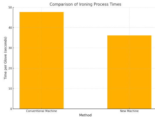
Fig. 5. Comparison of Ironing Process Times
